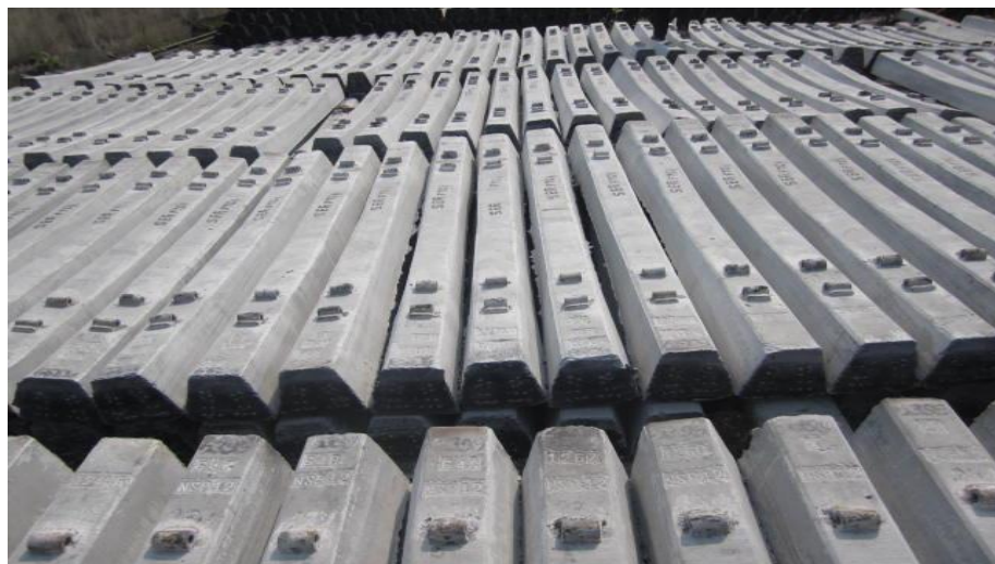
Rice.2. Basalt fiber in reinforced concrete sleepers.
