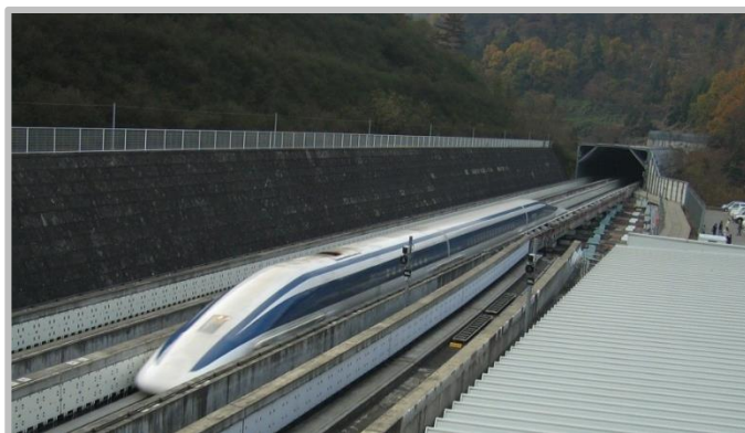
Figure 2 JR-Maglev high-speed Maglev train with magnetic suspension
